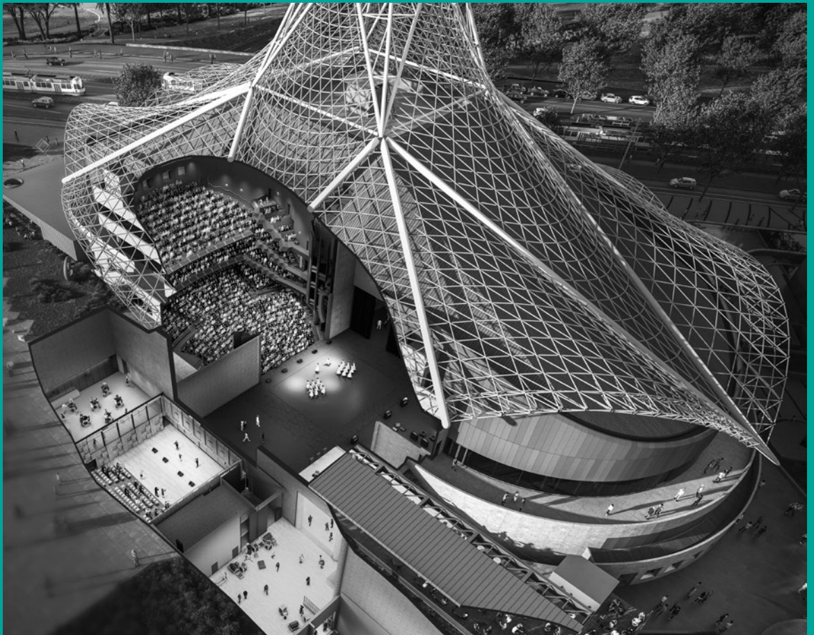
Concept-only render by NH Architecture showing extension of the Theatres Building basement structure, to provide a larger Loading Dock, new studio and rehearsal space, as well as a function room and new back-of-house spaces.
